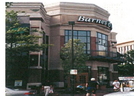
internally illuminated pan channel letters w/ acrylic faces
