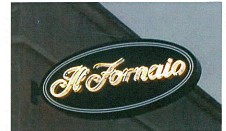
sign panel with exposed neon
