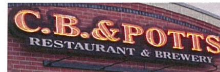
open pan channel letters with exposed neon
